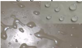
Hydrophobic and oleophobic display on this coatings surface
